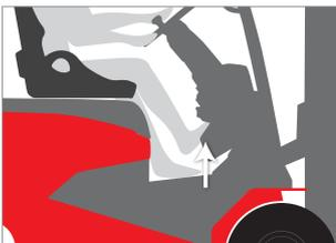
**Coasting:** Energy recovered when the foot is lifted off the accelerator.
