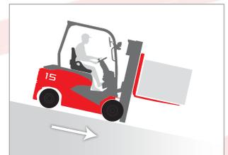
**Speed Suppression on Down-slope:** Energy recovered when cruising down-slope.
