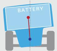
The small movement of the center of gravity during turning enables smooth and safe traveling.
