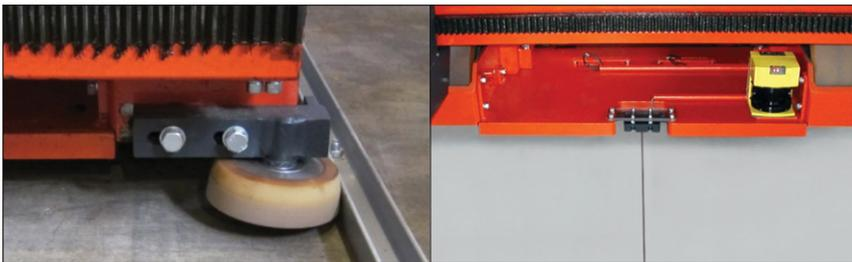
**Rail guidance rollers in standard or low profile:** height of profile minimum 38 mm      **Wire guidance**
